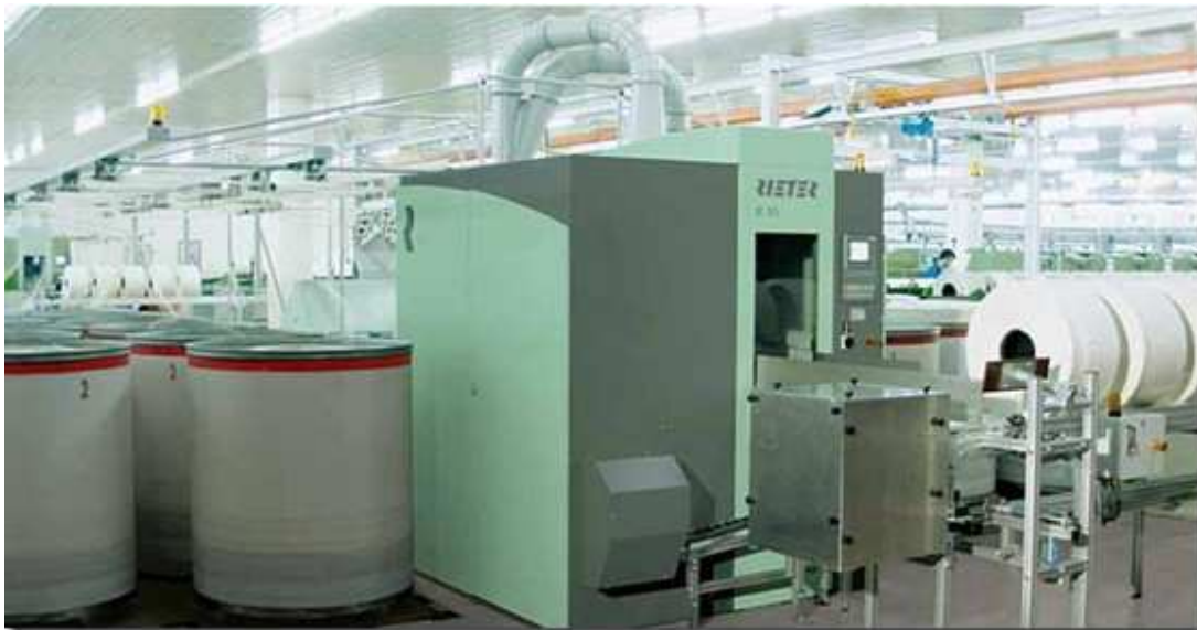
SERVOTrolley for semi-automatic lap transport
