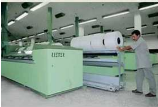
SERVOTrolley for semi-automatic lap transport
